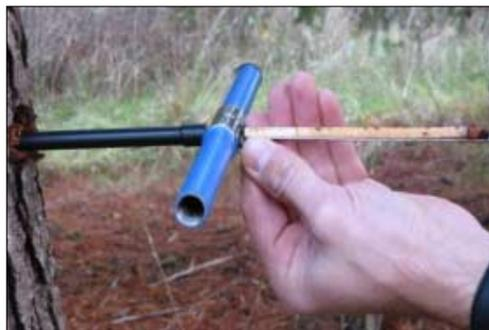
Figure 6.—A core sample obtained from a tree with the incremental borer enables the user to determine a tree's growth rate.
