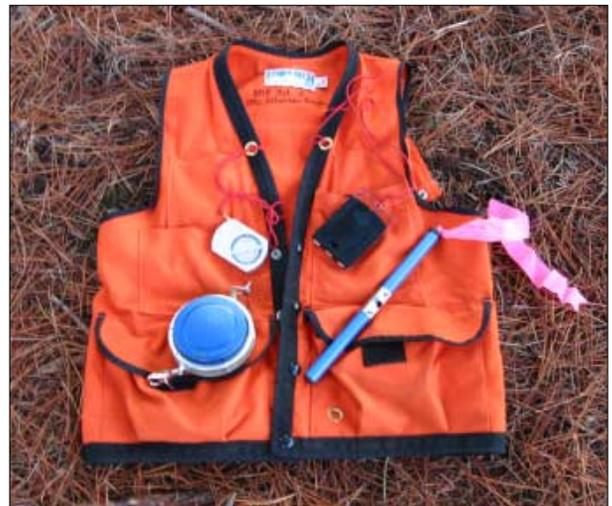
Figure 1.—Tools you'll use for some measuring tasks are (clockwise, from top left) a clinometer, a compass, an increment borer (with flagging tape attached, to make the borer easier to find if it falls on the ground), and a combination logger's tape.
