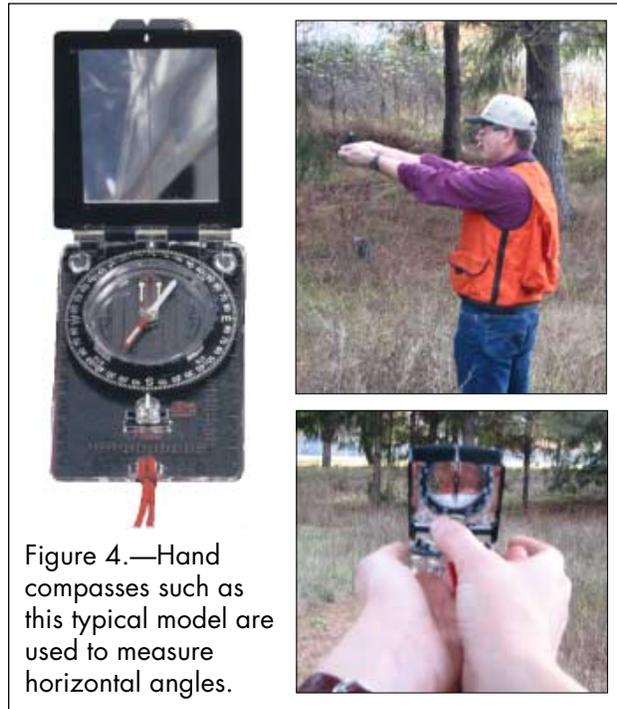
Figure 4.—Hand compasses such as this typical model are used to measure horizontal angles.
