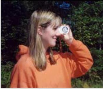
Figure 2.—The clinometer has a sighting hole and a suspended circular scale that can measure ground slope as well as tree height.
