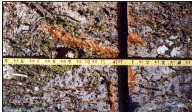
Figure 3.—A combination logger's tape can measure tree diameter (above left) in addition to log lengths and diameters (above right).
