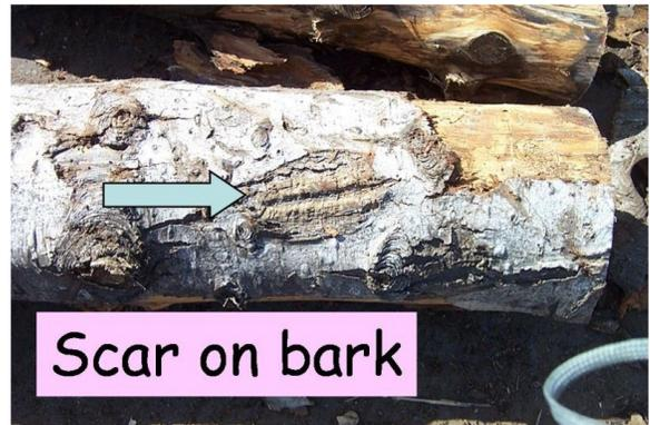
Inside the wood, this dead spot creates a weak area where there is no structural strength. Boards cut from trees with many of these unsuccessful attacks often fall apart due to the lack of structural integrity.
